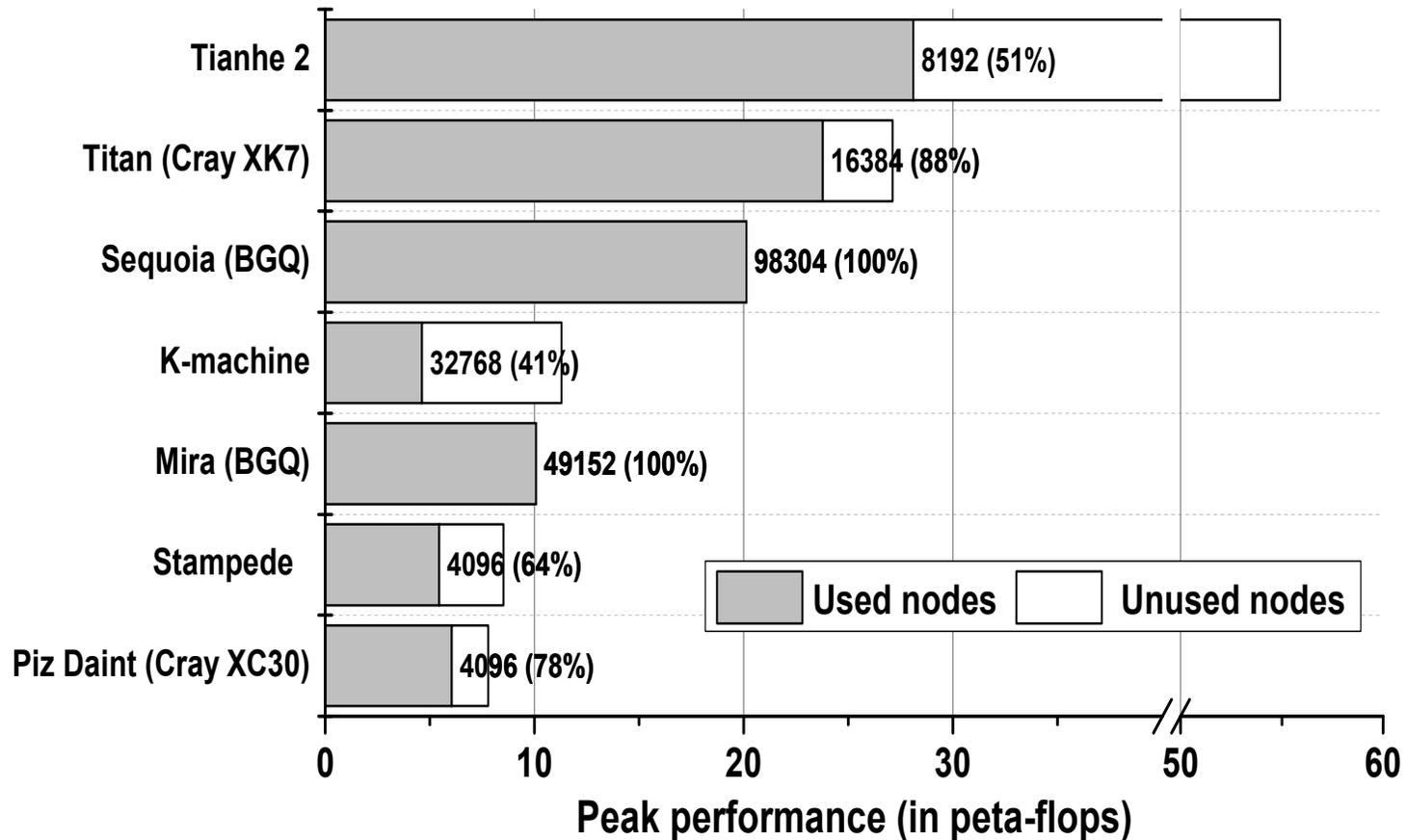
**Figure 1:** The GTC-P particle-in-cell (PIC) code has been ported to and optimized on a broad range of leading multi-petaflops supercomputers worldwide. Percentage indicates fraction of overall nodes utilized.
